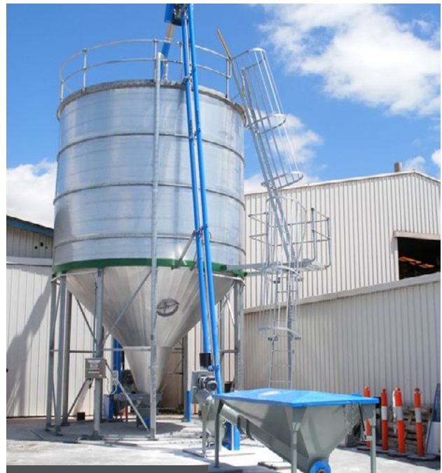
Floveyor feeding to Silo
